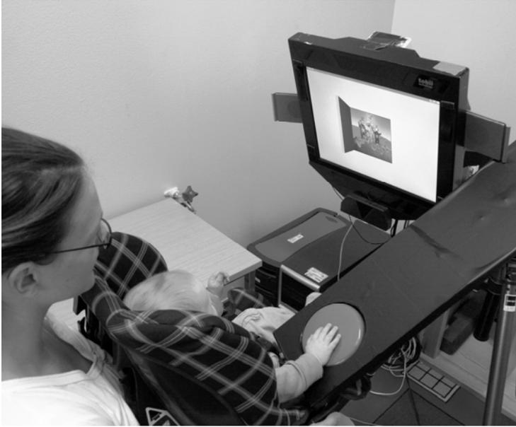
*Figure 2.* Photograph of the experimental setup, showing an infant seated in the safety car seat on the parent's lap, hand on button, watching video reward.
