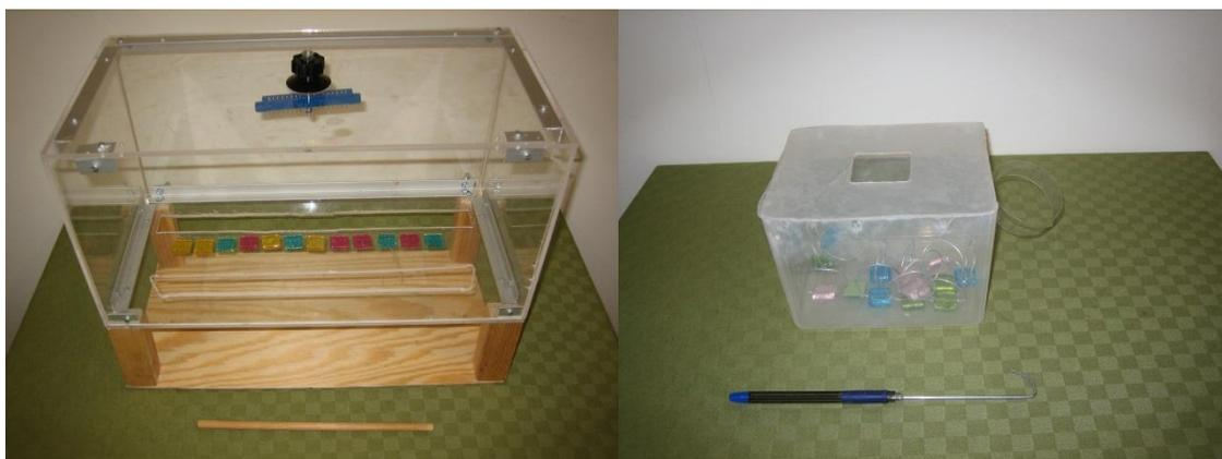
Figure 1. The push box (left) and the hook box (right), with pushing stick and hook.
